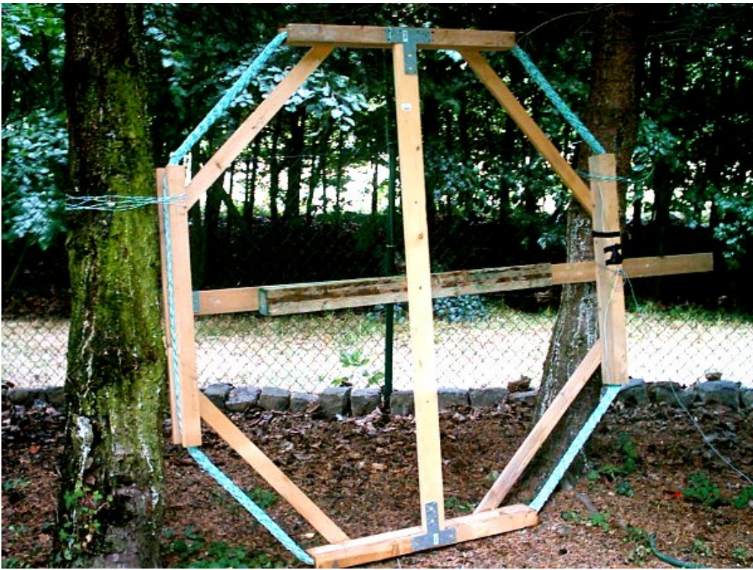
Coil Antenna with 400 turns, a diameter of 175 centimeters and a higher sensitivity than the described one
