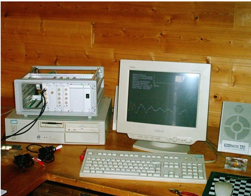
Analog ELF-receiver with connected PC and screen, showing a signal of type 2.
