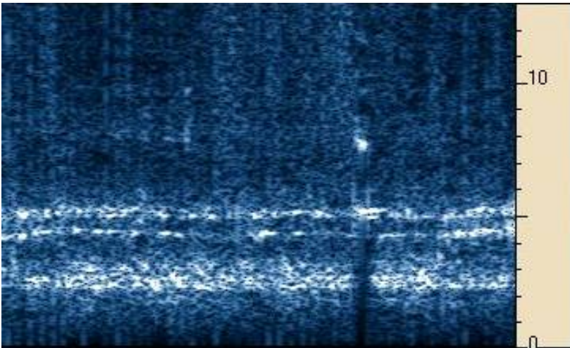
Spectrogram of 30', in 0-13 Hz band. Received with horizontal loop, 2100 sq.m. Analyzed with Spectran.
